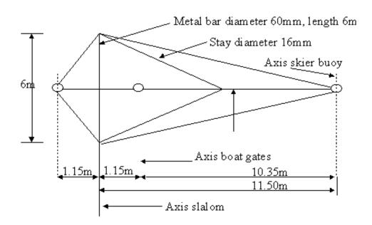
Diagram 9 - Handle measurement device dimensions
